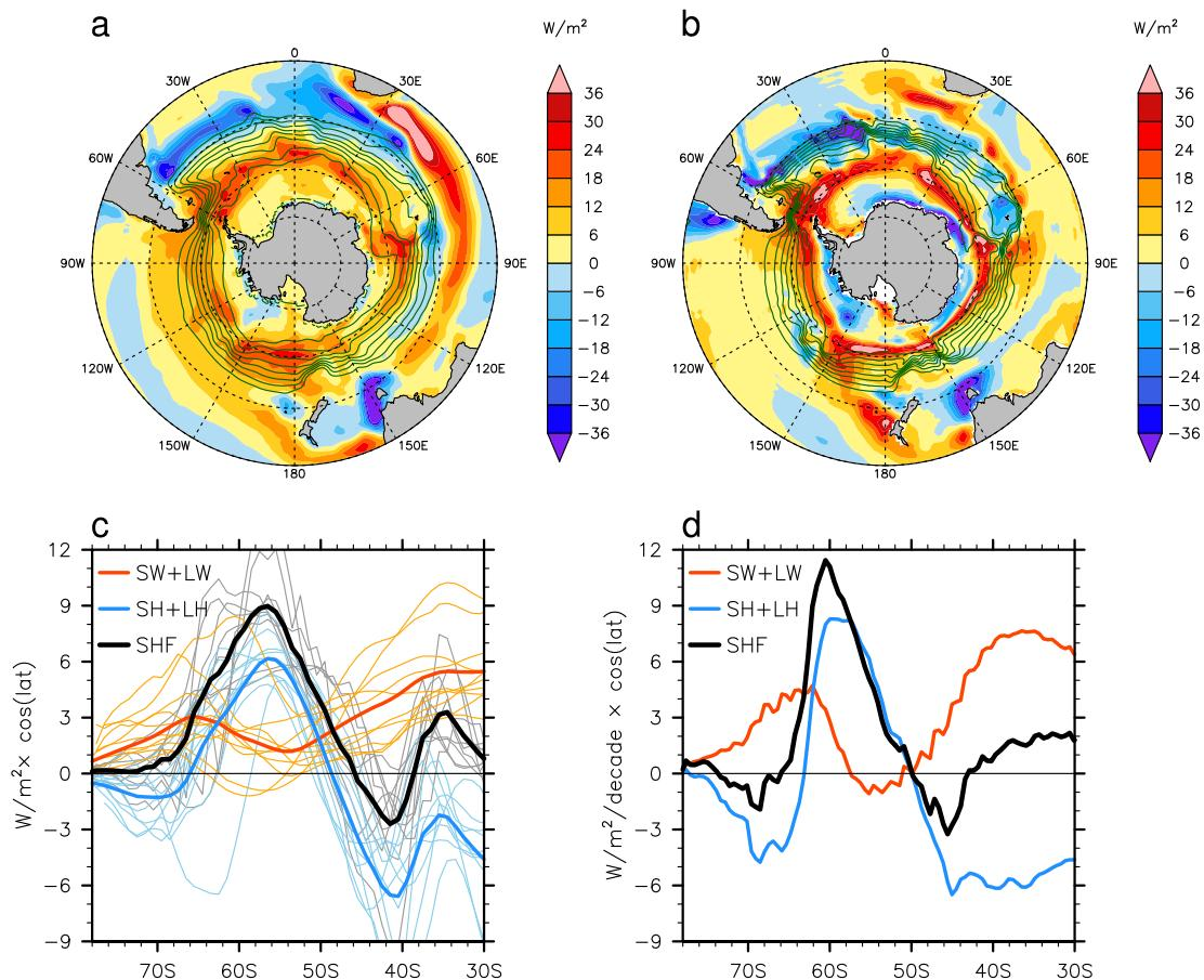
701 FIG. 1. Changes of net surface heat flux (*SHF*) over the Southern Ocean in response to quadrupled  $\text{CO}_2$
